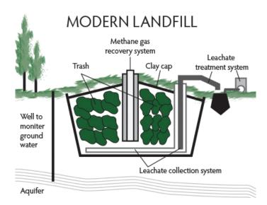
groundwater quality. A landfill is divided into a series of individual cells and only a few cells of the site are filled with trash at any one time. This minimizes exposure to wind and rain. The daily waste is spread and compacted to reduce the volume, a cover is then applied to reduce odours and keep out pests. When the landfill has reached its capacity, it is capped with an impermeable seal which is typically composed of clay soil.
