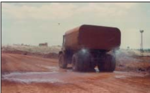
Water Sprinkler at Mine, NALCO
