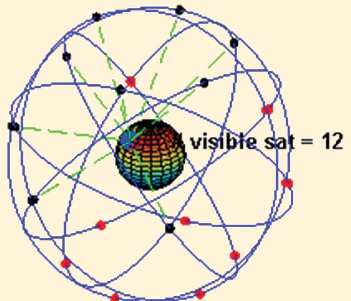
*24 satellite GPS constellation in motion with the Earth rotating 6 Orbits and 4 satellites in each orbit*
